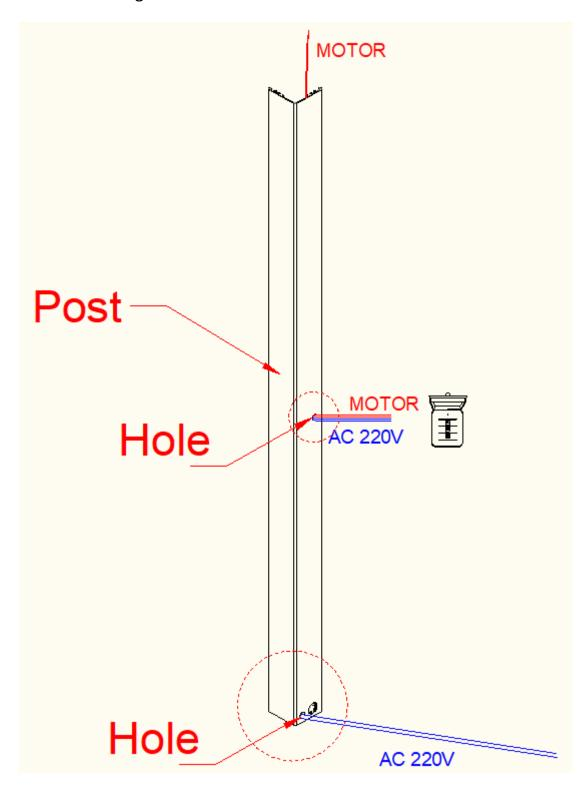
Not on the post, a location the customer wants. Just drill a hole in the post, as shown in the image below
